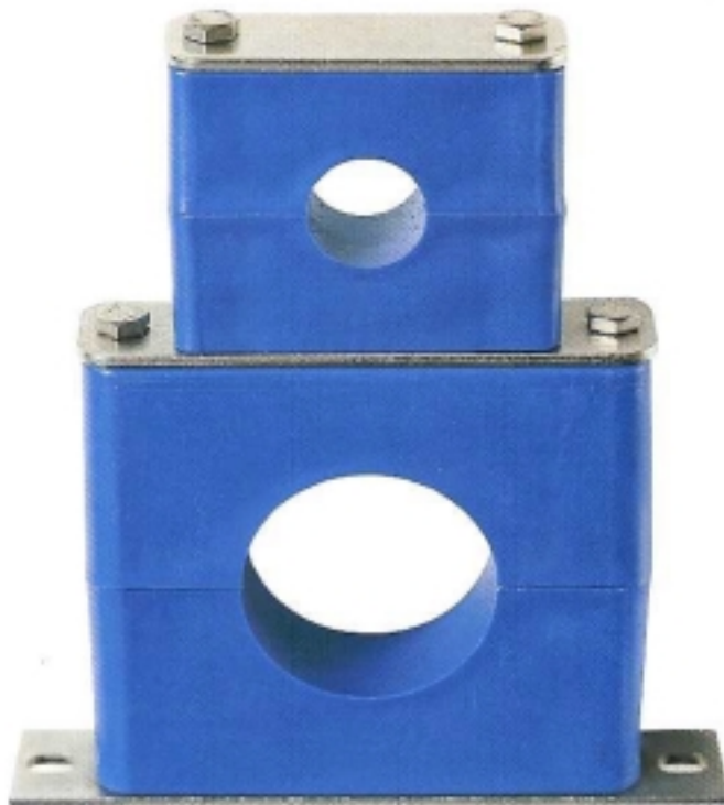
FIG 1: Transfer Plate allows vertical stacking of Behringer clamps to be easily accomplished for clamps of the same or different group sizes. Stacking bolts are used for clamps of the same group while a transfer plate connects clamps of different groups.
